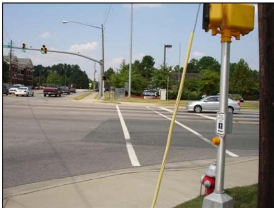
**Image 5-2.** The pedestrian crossing at the Kildaire Farm and Maynard Road intersection. Note the marked crosswalk and pedestrian-activated signals. These are standard features which should be installed with each new signal.
