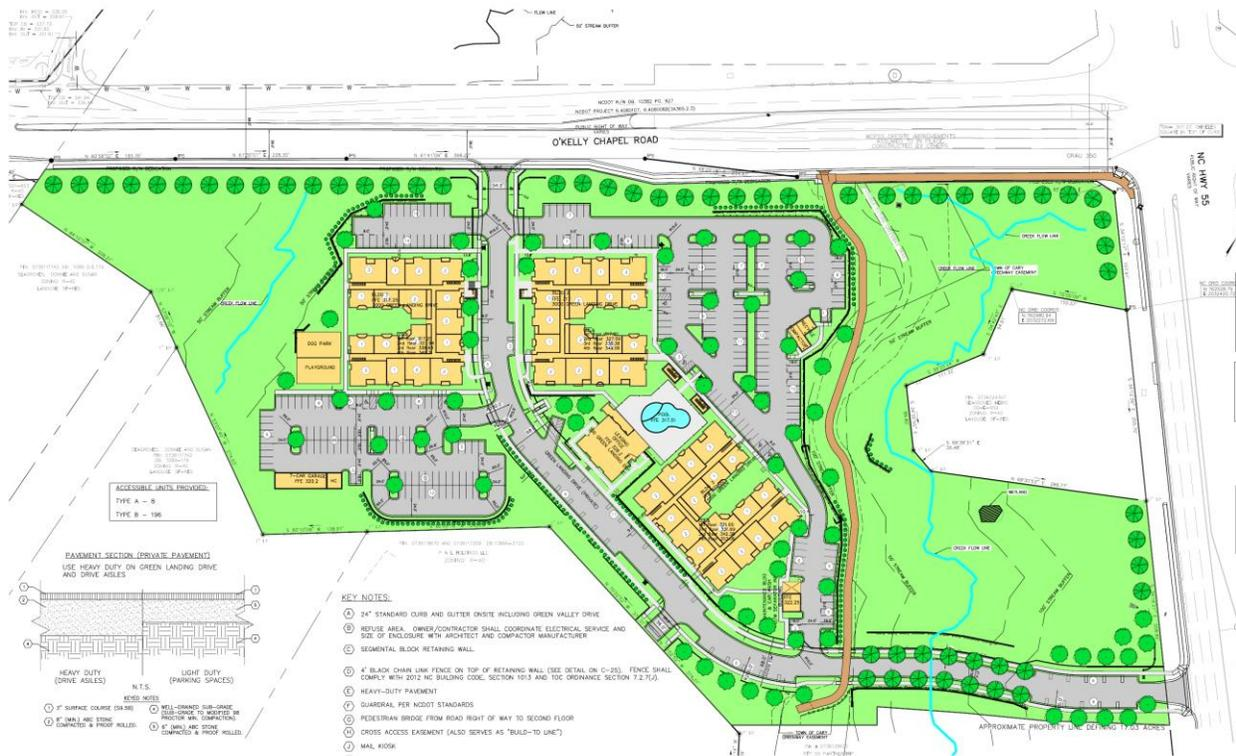
The development includes 204 units across three buildings. All three buildings are four stories high and front the private street. The two eastern buildings frame a clubhouse/office and pool. The buildings are a traditional multi-family form using pitched roof. The exterior is a masonry base supporting upper floors of cementitious siding. Cultured stone will accent the stairwell entrances. The color palette uses a warm palette of reds and reddish tan tones.
